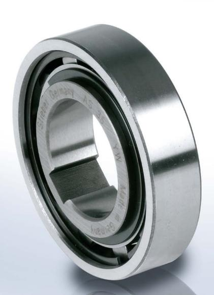
Type AS is a roller type freewheel non-bearing supported. Bearings are required to support axial and radial loads. Lubrication and sealing must also be provided by the installation. Nominal outside dimensions are the same as series 62.. ball bearings.
