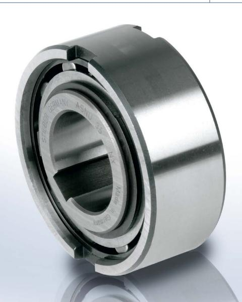
ype ASNU is a roller type freewheel non-bearing supported. Bearings are required to support axial and radial loads. Lubrication and sealing must also be provided by the installation. Nominal outer diameter is the same as a series 63.. ball bearing.
