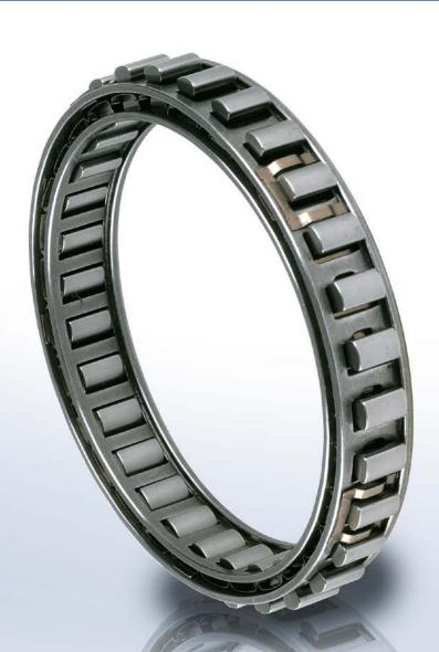
ype DC is a sprag type freewheel cage without inner or outer races. It must be installed in a design providing races, bearing support for axial and radial loads, lubrication and sealing. The DC type version-N accepts all types of lubricants currently used in the power transmission equipement.
