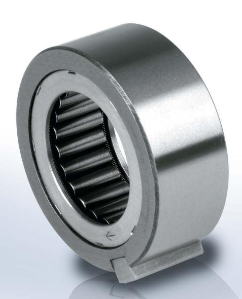
ype S200 is a non bearing supported sprag type freewheel. The sprags run directly on the shaft provided by the user. Bearings are required to support axial and radial loads. Lubrication and sealing must also be provided by the installation.
