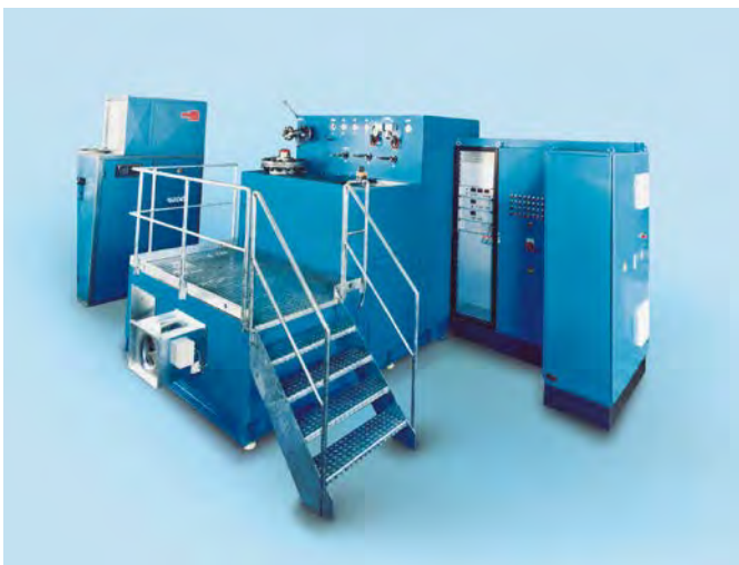
Test rig to determine pressure drop
