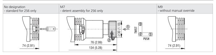
In case of solenoid malfunction or power failure, the spool of the valve can be shifted by manual override. For alternative manual overrides contact our technical support.
