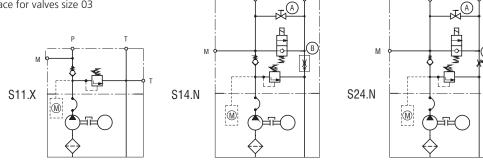
The hydraulic circuit S11.X enables the power pack to be used as a simple pressure supply for general applications with the possibility to build up additional hydraulic circuits in the form of horizontal stacking assemblies of the size 04 or 06 (S11.0) or size 03 (S11.1).
