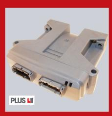
PLUS+1\* microcontrollers and I/O expansion modules are designed to provide flexible, expandable, and powerful machine management systems.
