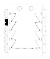
The flow rates of the adjacent outputs can be combined by plugging one or more outputs. In the example, by plugging output no. **8**, the lubricant passes on to the adjacent output (in the example, the number **6**) in a descending order. In case output no. **2** is plugged, the lubricant passes on to output no. **1**.
