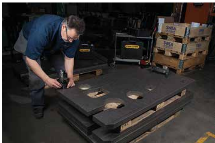
Flatness measurement of machine end after machining.
