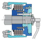
**Stromag KUK** as a basic type. For use outside gearboxes (dry operation). Hydraulic oil supplied axially through the shaft. Customer-specific adaptations of shaft and external body connections possible.
