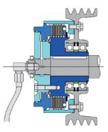
**Stromag KMK** as a shaft-pulley connection for use outside gearboxes (dry operation). Hydraulic oil can be supplied axially through the shaft. Available as a completely assembled and bearing supported unit.
