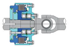
**Stromag KMK** for use in gearboxes (wet operation) with optional disc oil flushing. Hydraulic and cooling oil supplied via integrated radial oil supply (KRE).
