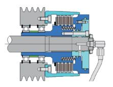
**Stromag KUK** as a shaft-pulley connection for use outside gearboxes (dry operation). Hydraulic oil supplied axially through the shaft. Available as a completely assembled and bearing supported unit.
