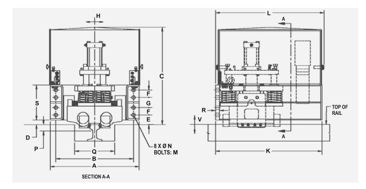
V Vertical Rail Deviation (Float) ±5mm relative to Rail Clamp enclosure at full rated capacity.
