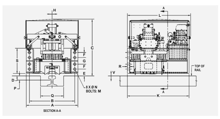
1V Vertical Rail Deviation (Float) ±25mm relative to Rail Clamp enclosure at full rated capacity.
