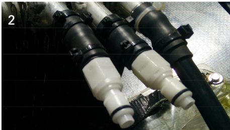
2 CPC Schnelltrenn-Kupplungen am Inverter und Grafikkarten Kühler. Gesponsored von wolftechnik Filtersysteme CPC quick-release couplings on the inverter and graphic card coolers. Sponsored by wolftechnik Filtersysteme
