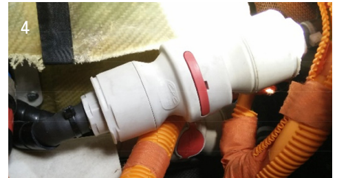
4 CPC Schnelltrenn-Kupplungen am Inverter. Gesponsored von wolftechnik Filtersysteme CPC quick-release couplings on the inverter. Sponsored by wolftechnik Filtersysteme
